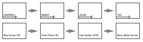
Adjust each function, CONTRAST, BRIGHTNESS, COLOR, TINT, ON/OFF, NTSC/PAL, NORMAL, MODE SELECTOR with VOL (+ -) button.
